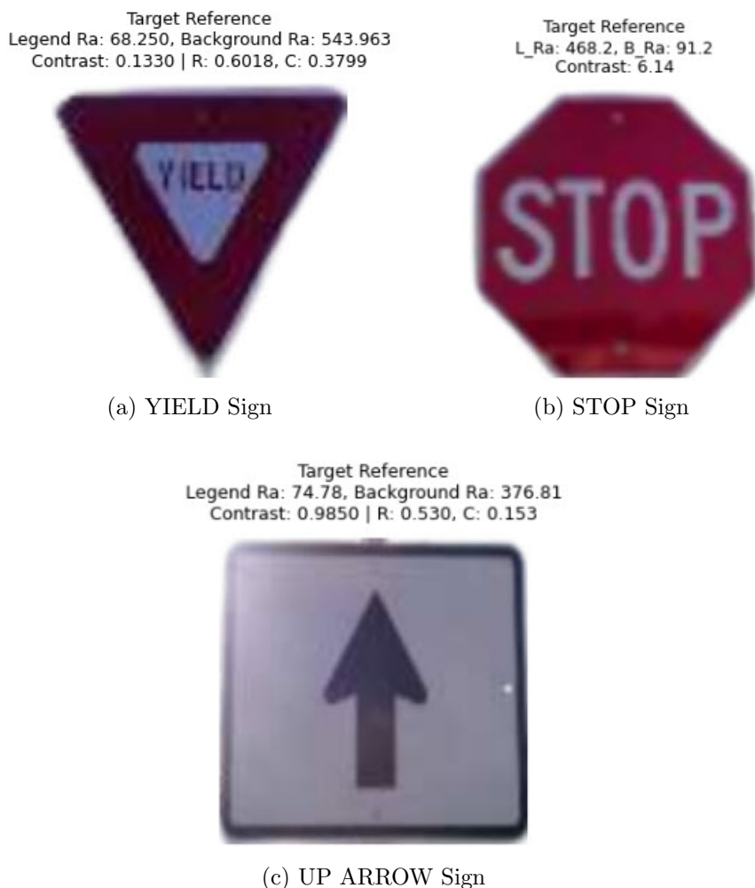
Figure 5.12: Real-world field dataset examples showing MUTCD compliance assessment. YIELD and ARROW signs demonstrate typical failure modes, while the STOP sign meets all federal thresholds. These examples illustrate the class imbalance challenge (2 of 3 unsafe) that requires synthetic data generation for balanced training.
